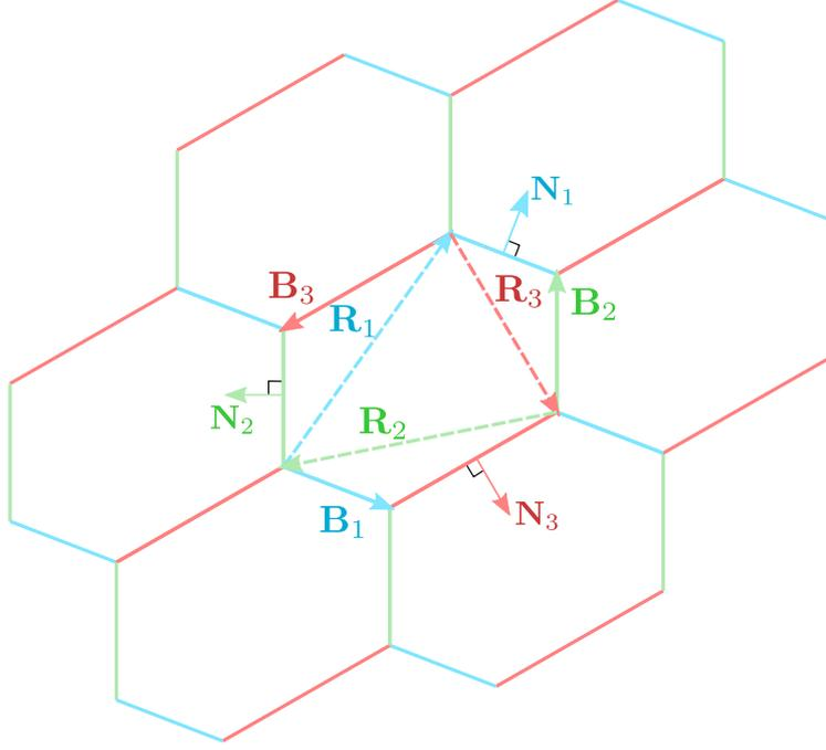
**Figure 2.** Periodic tiling of irregular hexagonal grains as considered by Wheeler [13]. Note that the centroid of each grain, and the midpoint of each grain boundary is a rotation centre of order two (the tiling is invariant under a rotation by  $180^\circ$  about these points). The symmetry of the tiling is the wallpaper group  $p2$ . All triple junctions in the tiling are indistinguishable owing to this symmetry.
